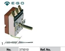
34352 thermostat  $t.max. 250^{\circ}C$  temperature range  $50\text{-}250^{\circ}C$  1-pole 1NO 16A probe ø 3.1mm probe L 208mm capillary pipe 1130mm capillary description pipe isolatedmm gland nut shaft L 23mm shaft position upper
