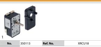
timer G 2-pole operation time 30min impulse mechanical 2NO at 250V 16A permanent position no shaft ø 3.5x3.5mm shaft 3.5x3.5mm shaft L 17mm mounting distance 28mm connection lateral
