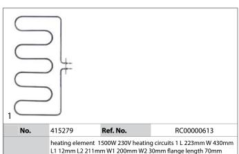
flange width 23mm hole distance 56mm tube ø 6.3mm windings 4
