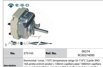
16A probe ø 6mm probe L 138mm capillary pipe 1480mm capillary pipe isolated 1100mm gland nut M9x1 shaft ø ø6x4.6mm shaft L 23mm shaft position upper rotation 270°
