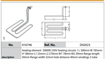
ø 8mm connection male faston 6.3mm hole ø 4.5mm rectangular
