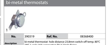
1NC 1-pole 16A connection F6.3 2 hole fixing
