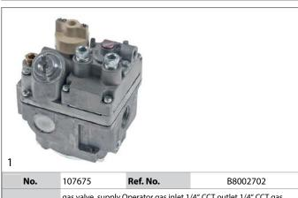
gas valve supply Operator gas inlet 1/4" CCT outlet 1/4" CCT gas inlet 1/2" NPT gas outlet 1/2" NPT thermocouple connection 11/32" pilot connection 1/4" CCT type 7000BGOR-LP pressure controller LPG 10"W.C.
