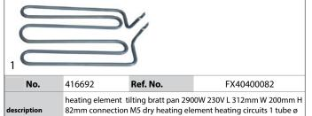
8.5mm W1 66mm W2 68mm connection distance 61mm
