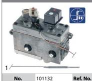
gas thermostat SIT type MINISIT 710 t.max. 340°C 100-340°C gas inlet 1/2" gas outlet 3/8" thermocouple connection M9x1 pilot connection M10x1 probe ø 5mm probe L 68mm capillary pipe 1050mm probe description type type B1 pressure controller no pressure regulatormbar gland nut ignition gas no
