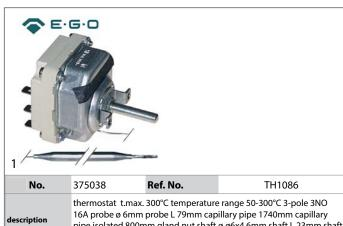
pipe isolated 800mm gland nut shaft ø ø6x4.6mm shaft L 23mm shaft position upper rotation 270°
