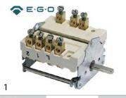
No.300103Ref. No.106062descriptioncam switch 4 operating positions 1NO/2CO sequence 0-1-2-3 32A shaft ø 6x4.6mm shaft L 23mm connection screw ceramic
