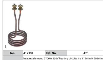
W1 44mm H1 160mm H2 45mm mounting distance 30mm thread 3/8" copper windings 4 tube ø 8.5mm immersion heater connection male faston 6.3mm
