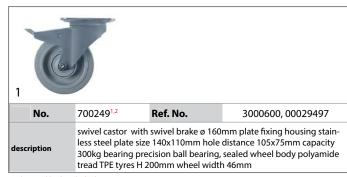
1with swivel brake 2hole distance 105x75 - 105x80
