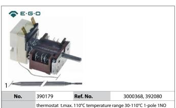
16A probe ø 6mm probe L 113mm capillary pipe 1430mm capillary
