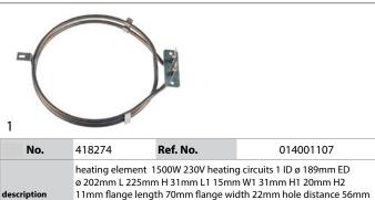
11mm flange length 70mm flange width 22mm hole distance 56mm connection male faston 6.3mm tube ø 6.5mm convection heating element hole ø 5mm rectangular flange
