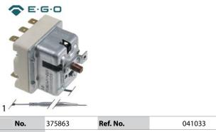
safety thermostat switch-off temp. 177°C 3-pole 20A probe ø 4mm probe L 128mm capillary pipe 2050mm capillary pipe isolated 2x110mm gland nut probe standard probe material SS
