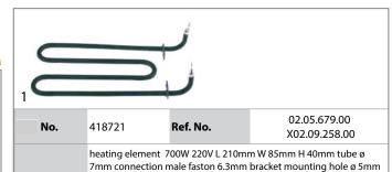
hole distance 66mm mounting distance 78mm heating circuits 1 lug length 25mm lug width 12.5mm dry heating element connection
