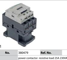
GR50-851000250 power contactor resistive load 25A 230VAC (AC3/400V) 9A/4kW main contacts 3NO auxiliary contacts 1NO/1NC connection screw description connection type LC1D09P7
