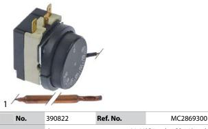
thermostat temperature range 30-90°C 1-pole 1CO 16A probe ø 6.5mm probe L 67mm capillary pipe 1450mm capillary pipe isolated description 70mm shaft ø 6x4.6mm shaft L 16mm shaft position lower rotation
