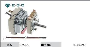
thermostat t.max. 470°C temperature range 100-470°C 1-pole 1NO 16A probe ø 3.9mm probe L 228mm capillary pipe 1110mm capillary description pipe isolated 600mm gland nut shaft ø ø6x4.6mm shaft L 24mm shaft position upper rotation 270° outer switch 2NO
