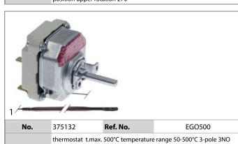
16A probe ø 4mm probe L 228mm capillary pipe 1200mm capillary
