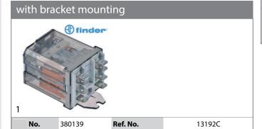
power relays FINDER 230VAC 16A 2CO connection F6.3 bracket mounting dimensions 68x38.2x35.8mm manuf. no. 62.82.8.230.0000
