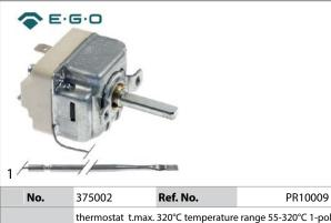
thermostat t.max. 320°C temperature range 55-320°C 1-pole 1NO 16A probe ø 3.1mm probe L 226mm capillary pipe 870mm capillary pipe isolated 850mm gland nut shaft L 23mm shaft position upper rotation 270°
