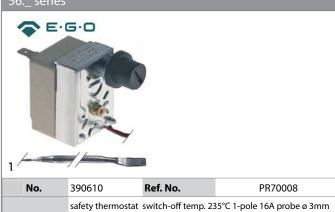
probe L 190mm capillary pipe 1000mm capillary pipe isolated
