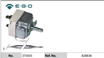
thermostat t.max. 110°C temperature range 30-110°C 1-pole 1CO 16A probe ø 6mm probe L 130mm capillary pipe 1500mm capillary pipe isolatedmm gland nut shaft L 23mm shaft position upper rotation 318° 250V
