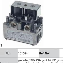
gas valve 230V 50Hz gas inlet 1/2" gas outlet 1/2" pilot connection level slow ignition standard ignition time 3-7s pressure range 3-50mbar power supply for modulator type SIT equiv. no. 0.830.034
