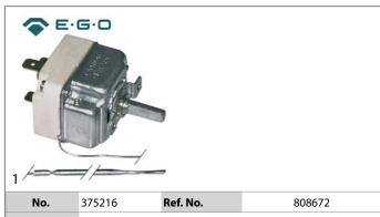
thermostat t.max. 280°C temperature range 50-280°C 1-pole 1NO
