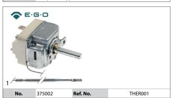
thermostat  $t.max. 320^{\circ}C$  temperature range 55-320 $^{\circ}C$  1-pole 1NO 16A probe ø 3.1mm probe L 226mm capillary pipe 870mm capillary
