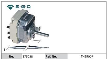
thermostat t.max. 300°C temperature range 50-300°C 3-pole 3NO 16A probe ø 6mm probe L 79mm capillary pipe 1740mm capillary description pipe isolated 800mm gland nut shaft ø ø6x4.6mm shaft L 23mm shaft position upper rotation 270°
