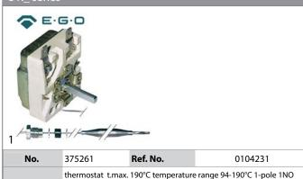
15A probe ø 6mm probe L 133mm capillary pipe 890mm capillary
