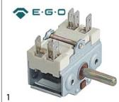
300129 No. Ref. No. 09/1324 cam switch 2 operating positions 2NO sequence 0-1 16A shaft ø description 6x4.6mm shaft L 23mm connection male faston 6.3mm ceramic
