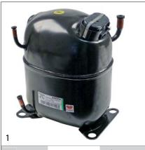
No. 605190 Ref. No. 092906 compressor coolant R404a/R507 type NJ9232GK 220-240V 50Hz HMBP 22.1kg 1 1/4HP cylinder capacity 26.2cm<sup>3</sup> CSR H 277mmWW description 1093W 1470W 1911W 2413W 2973W 3588W 4255W ambient temperature max. 45°C
