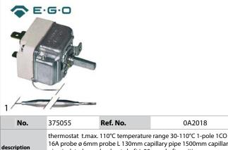
16A probe ø 6mm probe L 130mm capillary pipe 1500mm capillary pipe isolatedmm gland nut shaft L 23mm shaft position upper
