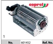
300778 cross flow fan TFL 180 roller ø 60mm roller length 180mm laminated core thickness 20mm motor position left 230V/50Hz 19W universal description bearing silicone connection male faston 6.3mm airflow 100m<sup>3</sup>/h -30 up to +100°C 230V 50Hz
