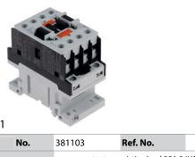
power contactor resistive load 25A 24VAC (AC3/400V) 9A/4.2kW main contacts 4NO auxiliary contacts connection screw connection type BF09T4A024
